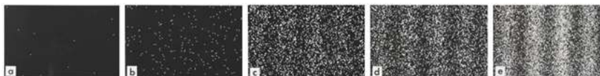
The double slit experiment with electrons: a) 10 electrons; b) 100; c) 3,000; d) 20,000; e) 70,000 electrons.
